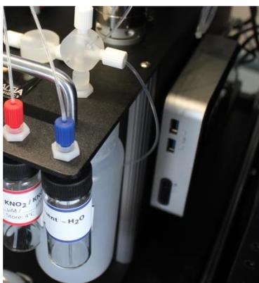
The software is installed on an Intel NUC computer which is mounted on the side of the FloPro. This compact computer is equipped with a 4<sup>th</sup> Gen Intel i5 processor and Windows 7 operating system. It's built in Wi-Fi means that the computer is accessible wherever Internet connectivity is available.
